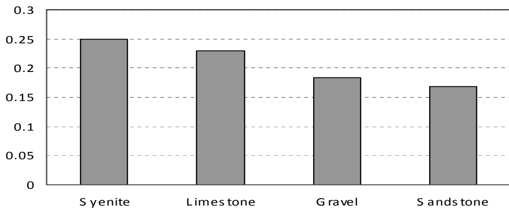
Figure 20 Effect of Aggregate Type on Poisson's Ratio
