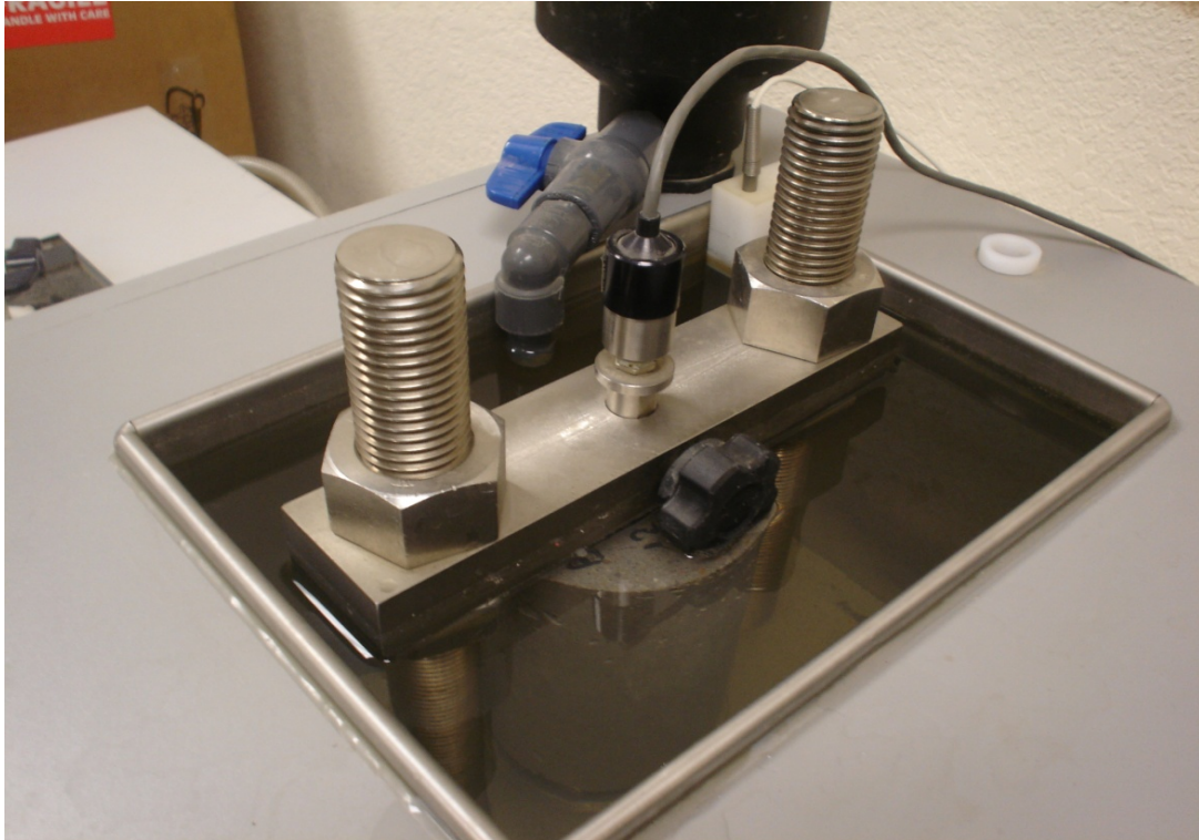
Figure 8 CTE Test setup showing specimen in water bath attached to LVDT (8).
